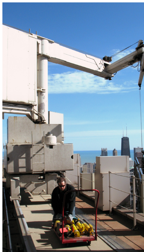
Preparing to weigh building maintenance unit to determine the loads on the track system.
