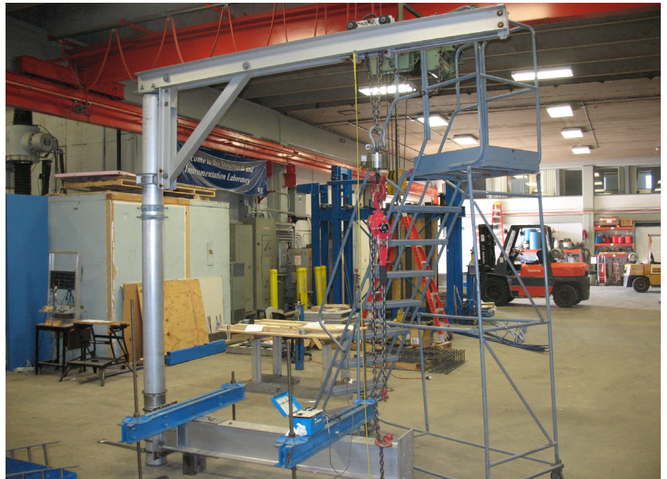
Testing of davit arm in WJE structural laboratory.
