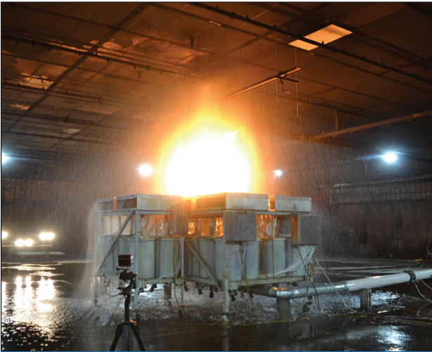
This project was unique due to the innovative use of the actual delivered density apparatus as a scoping tool for full-scale testing, which provides a methodology to identify trends and identify scenarios that may pass or fail the selected performance criteria. Photo: Wiss, Janney, Elstner Associates, Inc.
