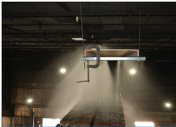
Early suppression fast response sprinkler technology was introduced in the late 1980s. Photo: Wiss, Janney, Elstner Associates, Inc.
